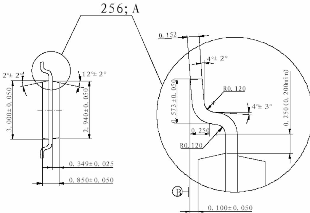
Figure 8 VA7205 8-Pin MSOP Mechanical Date (unit: mm unless otherwise specified)
