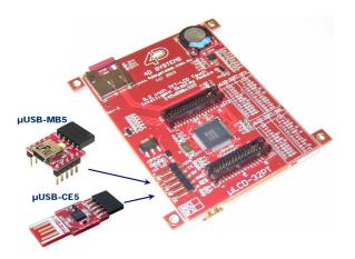
The PmmC file is programmed into the device with the aid of "*PmmC Loader*", a PC based software tool. To provide a link between the PC and the ICSP interface a USB to Serial converter is required. A range of custom made micro-USB devices such as the uUSB-MB5 and the uUSB-CE5 are available from 4D Systems.
