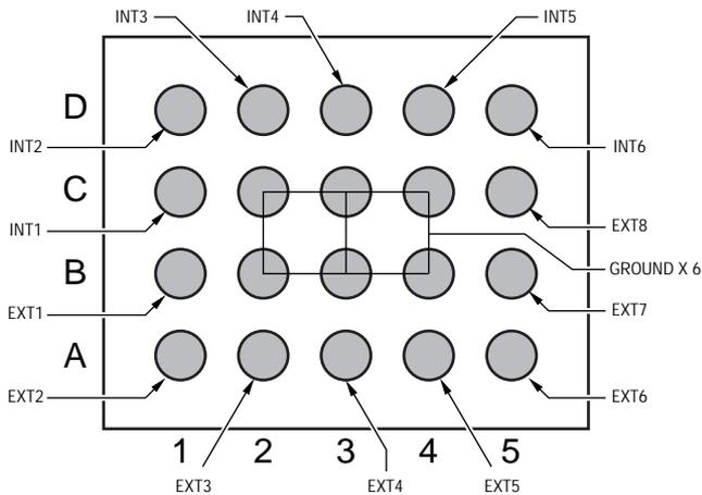
Fig. 6 (a) - Device Pin Out "Bumps Up" View
