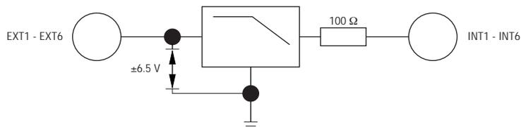
Fig. 3 - Channel Schematic
