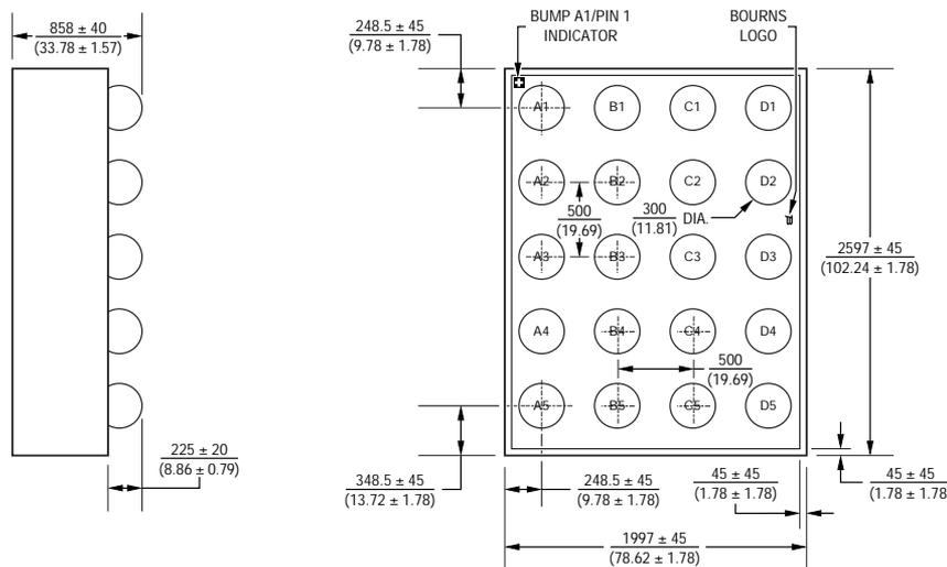
Fig. 2 - Device Mechanical Drawing
