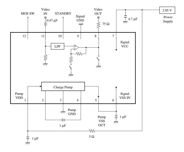
Note) The Above circuit and peripheral part's constants shows an example of design, but it is not guaranteed as those for mass production sets.
