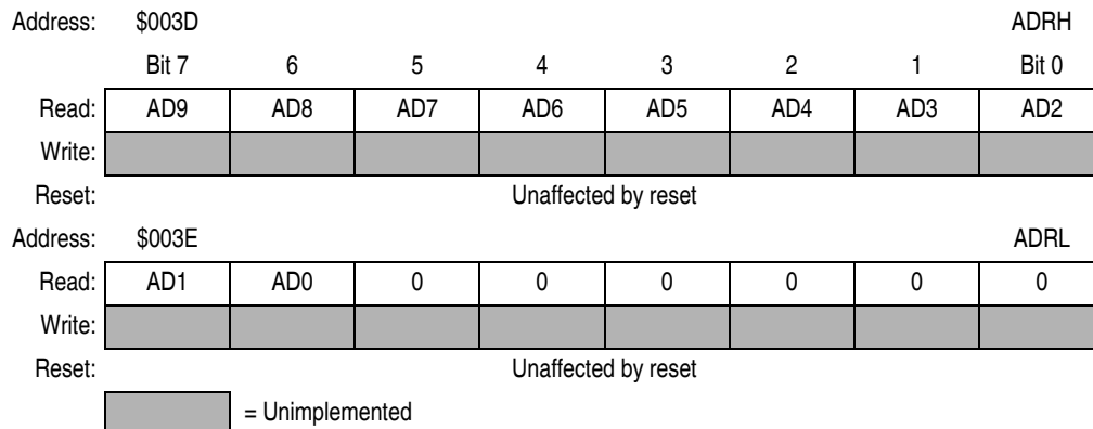
Figure 3-5. ADC Data Register High (ADRH) and Low (ADRL)
