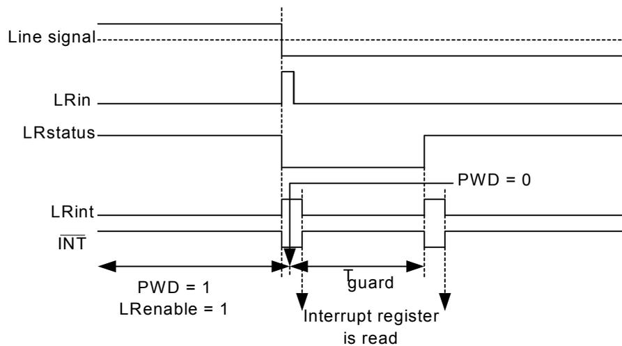
Figure 12 : Behavior of signals on a line reversal
