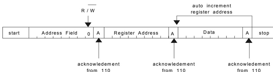
Figure 27: Write sequence of the serial interface
