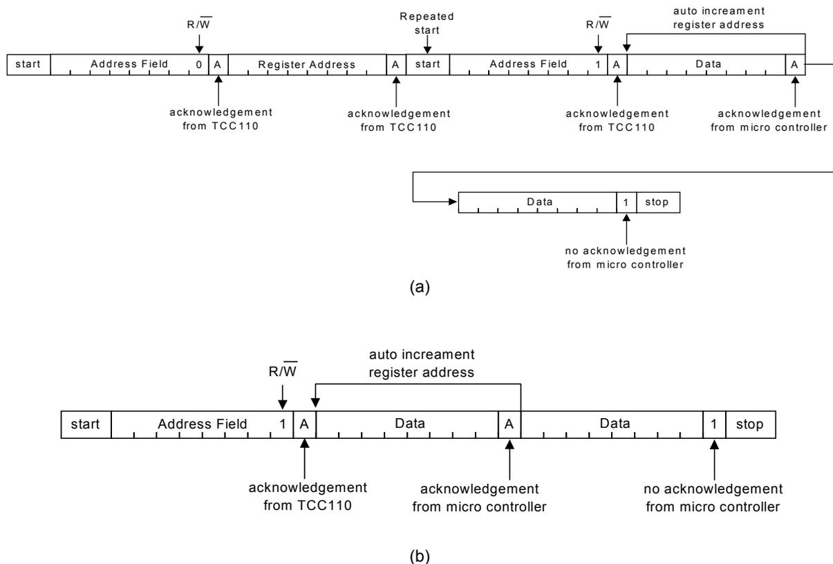
Figure 28: Read sequence of the serial interface
