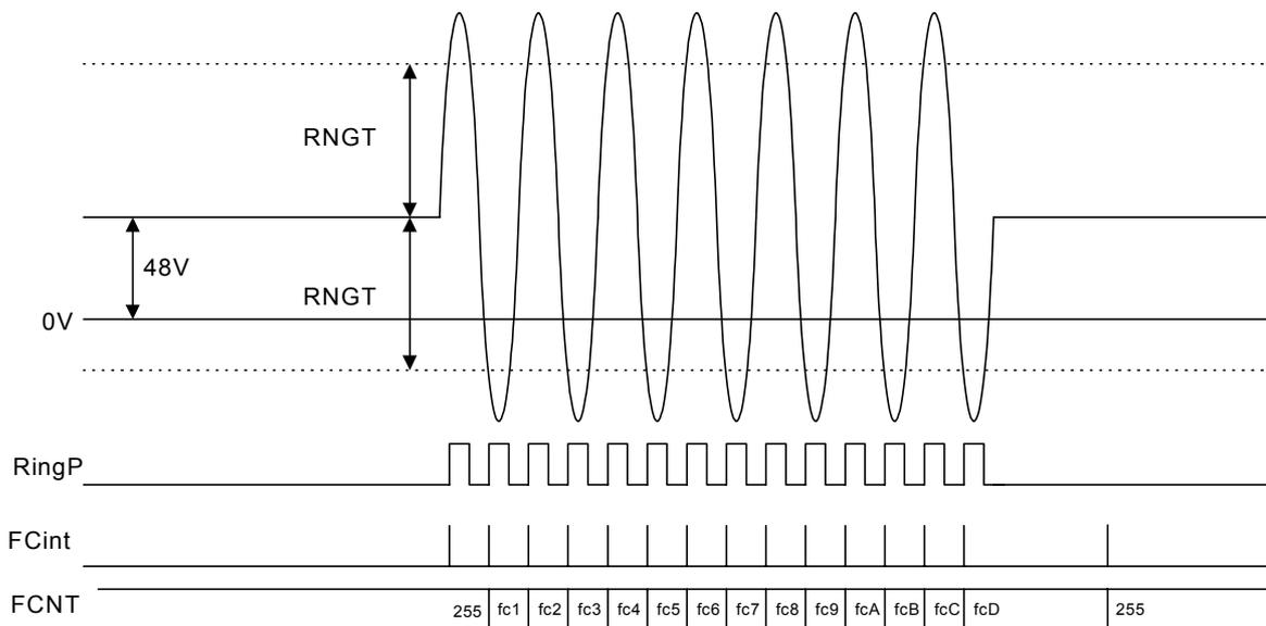
Figure 21: Behavior of RING when a ring occurs on the line
