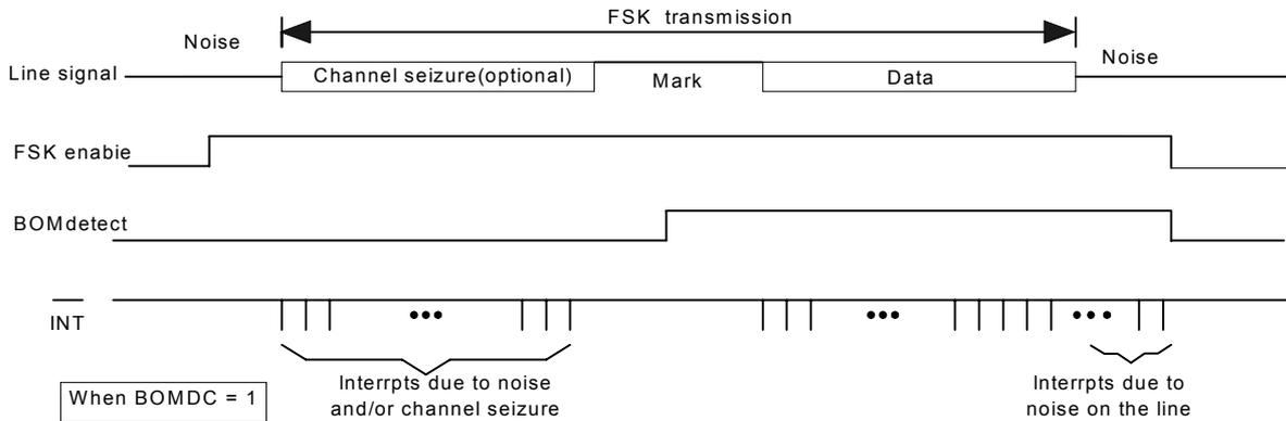
Figure 8: Interrupt behavior of the FSK receiver with BOMDC = 1
