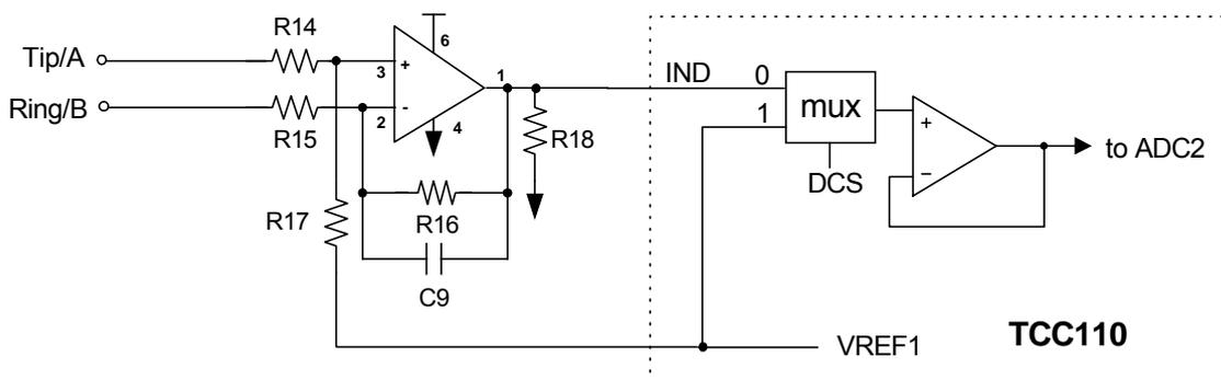
Figure 5. DC input buffer of the TCC110
