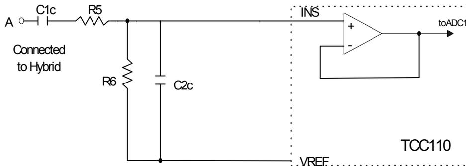
Figure 4. Single ended buffer of the TCC110
