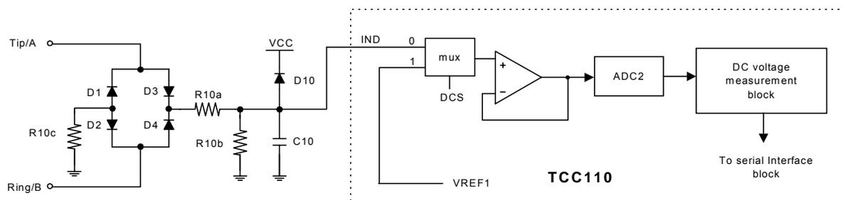
Figure 14: DC voltage measurement block
