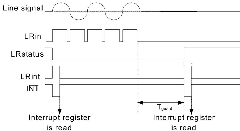
Figure 13: Behavior of signals during ring
