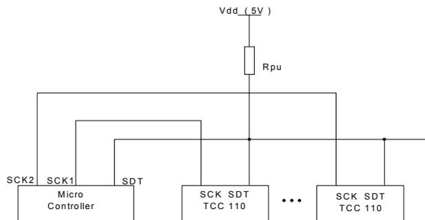
Figure 22: Serial bus configuration
