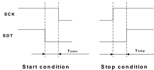
Figure 32: Timing constraints of start and stop conditions
