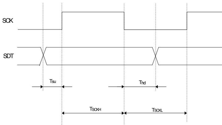
Figure 33: Timing of SCK and SDT during byte transmission
