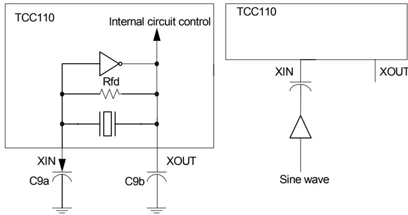
Figure 29: (a) oscillator with external capacitor (b) External clock: sine wave
