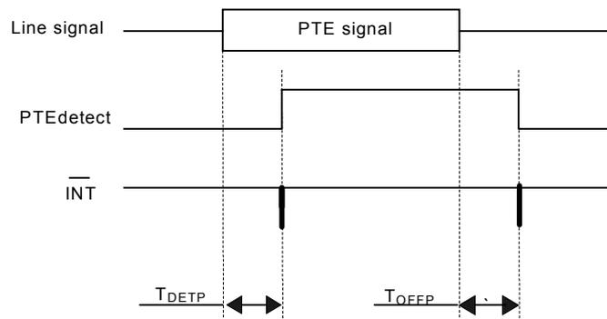
Figure 31: Timing of the PTE detection signals related to the progress tone
