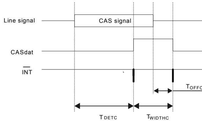
Figure 30: Timing of the CAS detection signals related to the CAS tone
