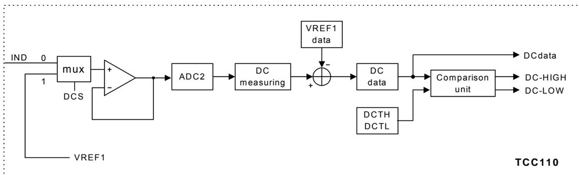
Figure 18: DC measurement block configuration for DC line voltage measurement mode
