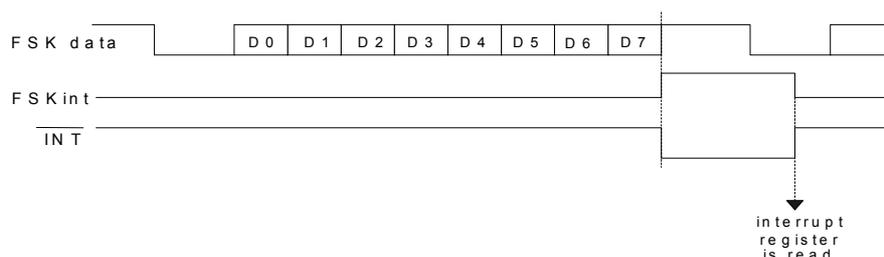
Figure 7. Sequence to receive an FSK data byte
