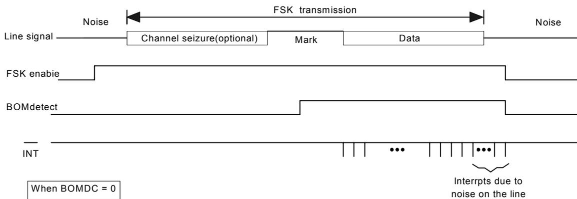
Figure 9: Interrupt behavior of the FSK receiver with BOMDC = 0
