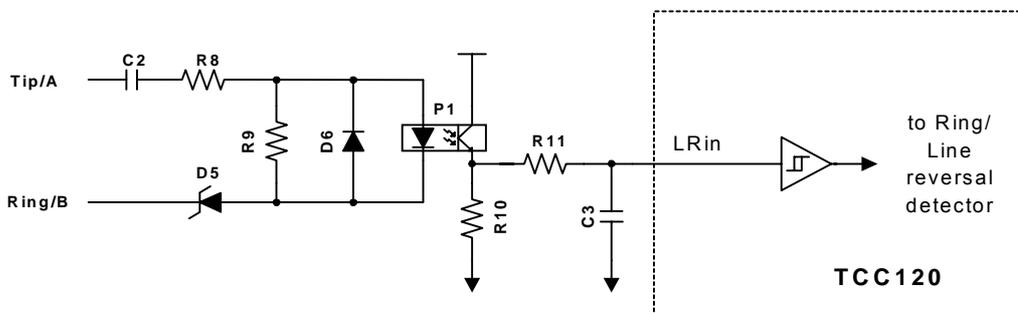
Figure 11. External component to generate LRin
