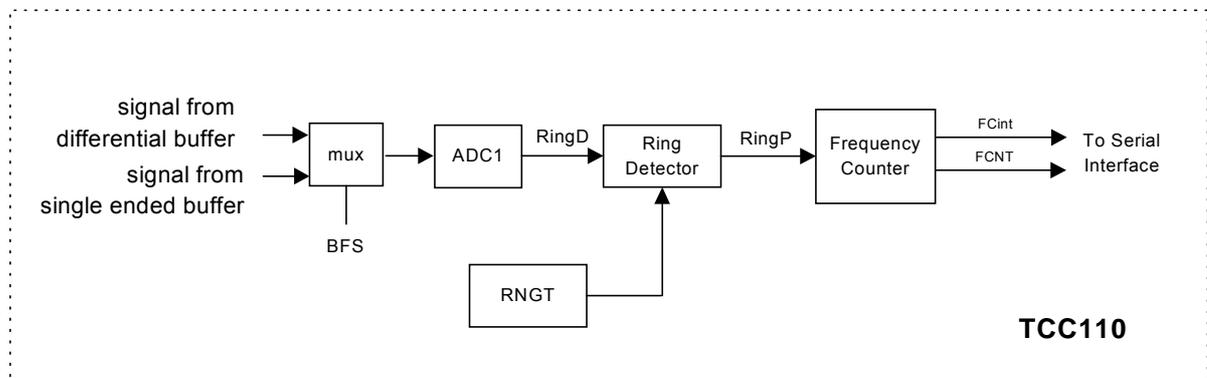
Figure 20: Ring detection and frequency counting block
