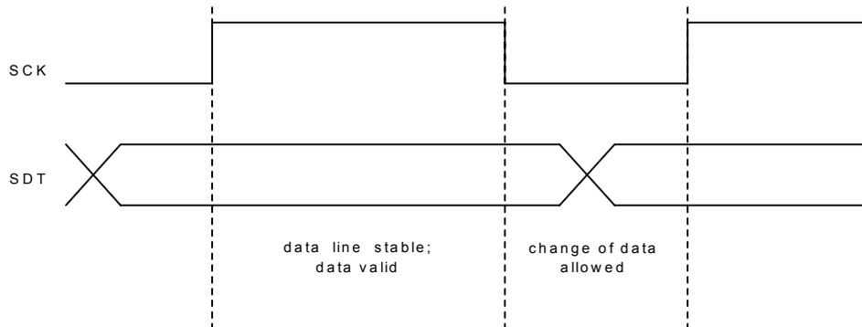
Figure 24. Bit transfer timing
