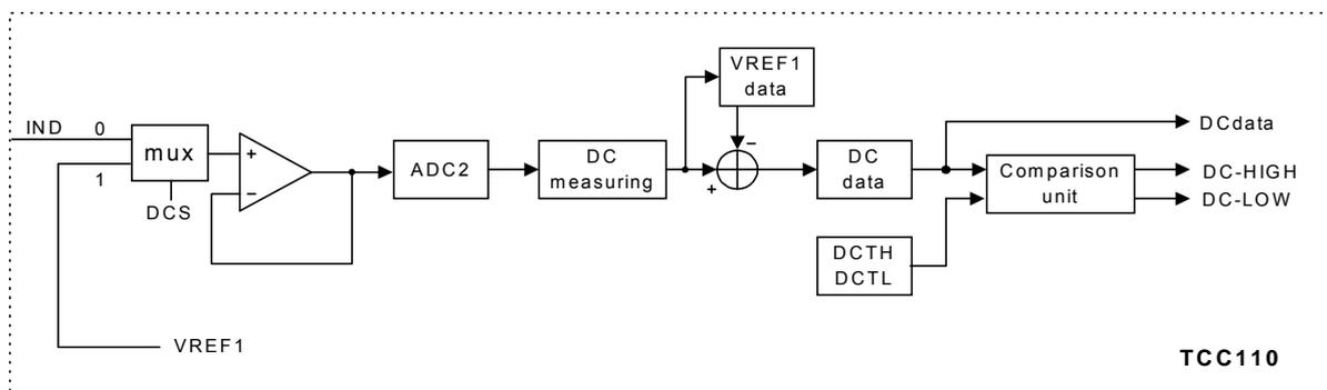
Figure 19: DC Level Detector configuration for reference voltage measurement mode
