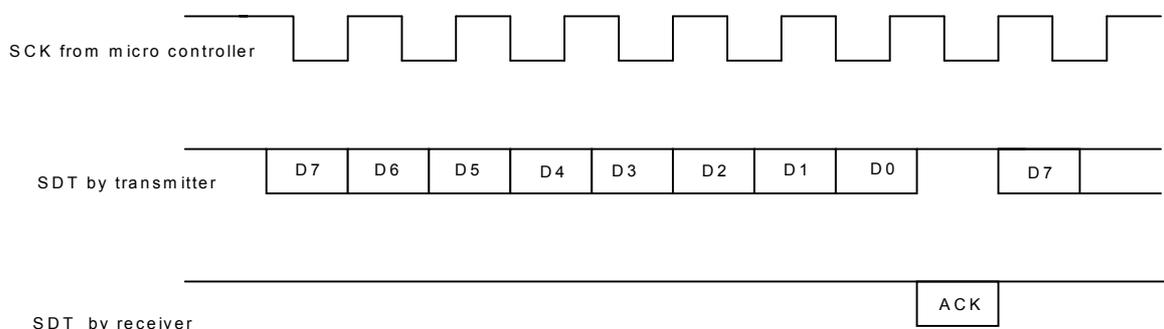
Figure 25. Byte transmission and acknowledge
