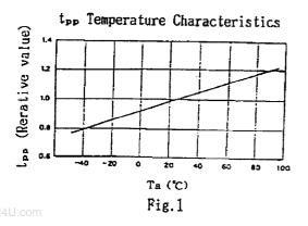
BUSY Pin Output Delay Characteristics
