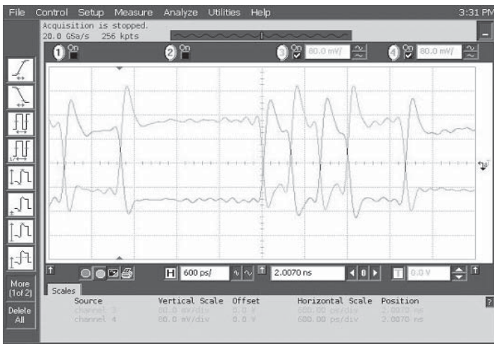
Data Waveforms, 2.5Gbps (left) & 5.0Gbps (right)
