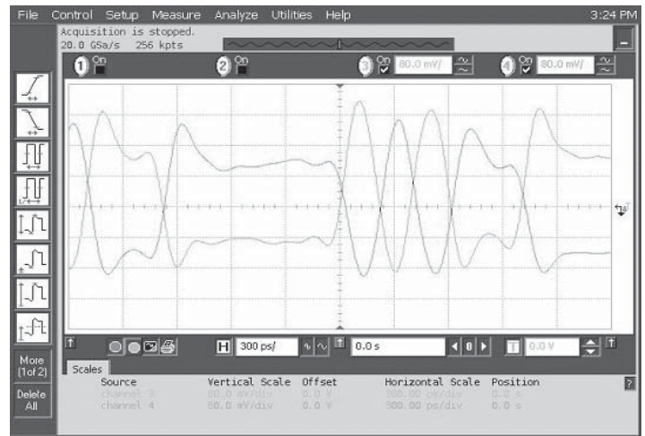
Data Waveforms, 2.5Gbps (left) & 5.0Gbps (right)
