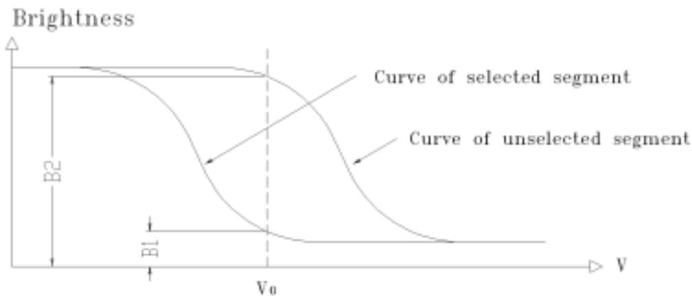
$$\text{Contrast Ratio} = B2/B1 = \frac{\text{unselected state brightness}}{\text{selected state brightness}}$$
