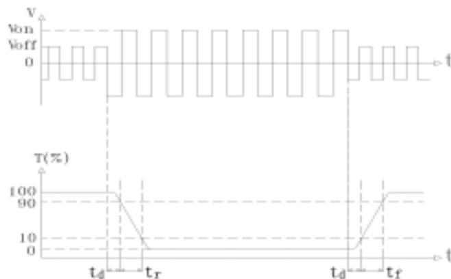
Turn on time:  $t_{on} = t_d + t_r$
