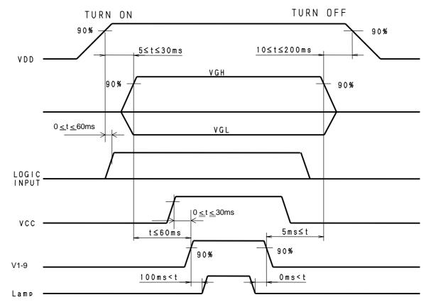
Turn on :VDD $\rightarrow$ VGL $\rightarrow$  VGH $\rightarrow$ Logic input $\rightarrow$ VCC $\rightarrow$  V1-V9 Turn off :V1-V9 $\rightarrow$  VCC $\rightarrow$ Logic input $\rightarrow$ VGH $\rightarrow$  VGL $\rightarrow$  VDD
