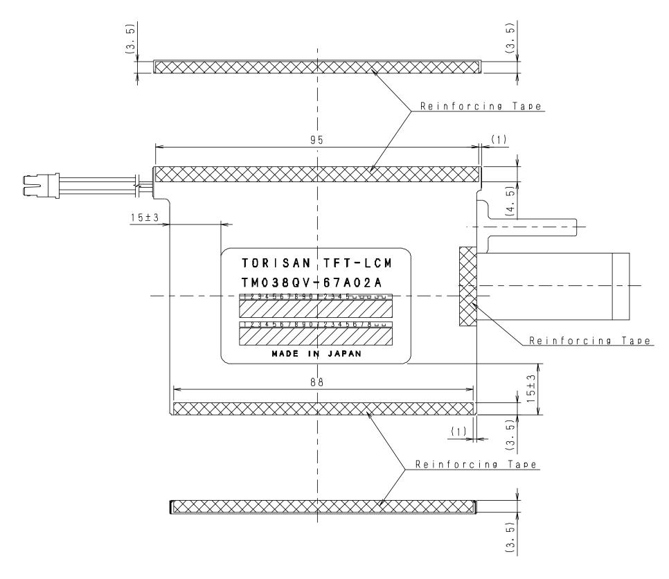
Note1:Unspecified dimension tolerances are  $\pm 0.5\,\text{mm}$ .
