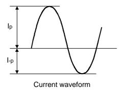
Unbalance rate =  $| I_p - I_{-p} | / I_L \times 100$  (%) Wave-height rate =  $I_p$  (or  $I_{-p}$ ) /  $I_L$
