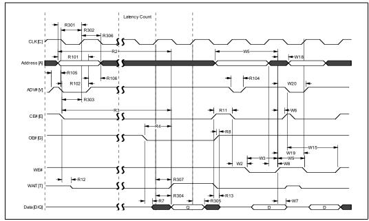
Figure 20. Synchronous Write To Read Operation
