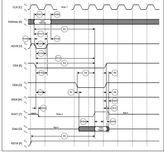
Figure 11. Single Synchronous Read-Array Operation Waveform
