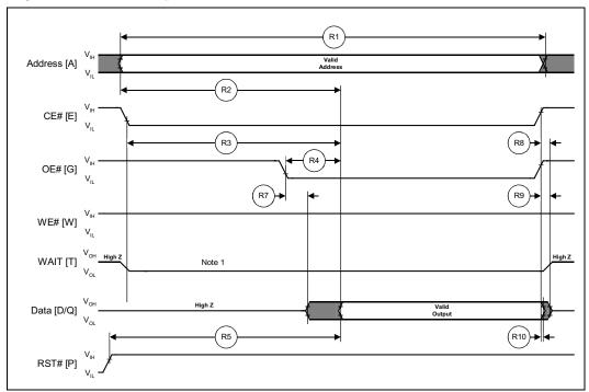
Figure 8. Asynchronous Read Operation Waveform
