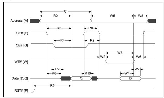
Figure 17. Asynchronous Read to Write Operation Waveform
