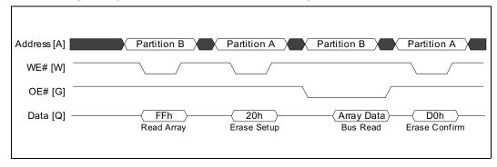
By contrast, a write bus cycle may not interrupt a 2-cycle write sequence. Doing so causes a command sequence error to appear in the status register. Figure 27 illustrates a command sequence error.
