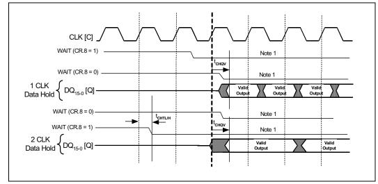
Figure 41. Data Output Configuration with WAIT Signal Delay
