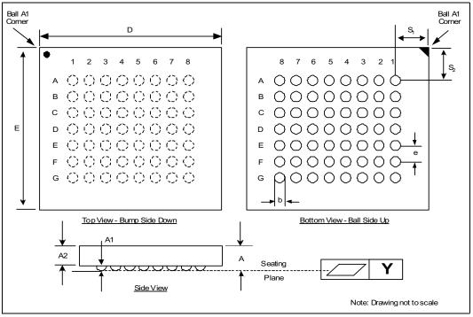
Figure 3. 128-Mb VF BGA Package Drawing
