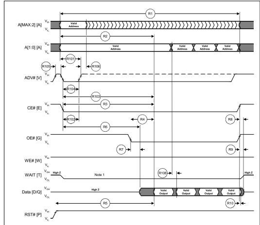
Figure 10. Page-Mode Read Operation Waveform
