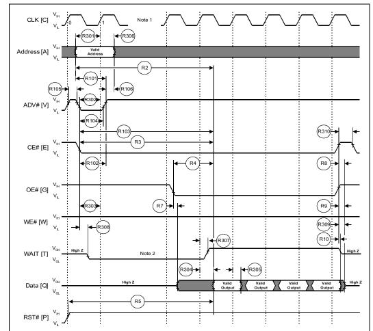
Figure 12. Synchronous 4-Word Burst Read Operation Waveform
