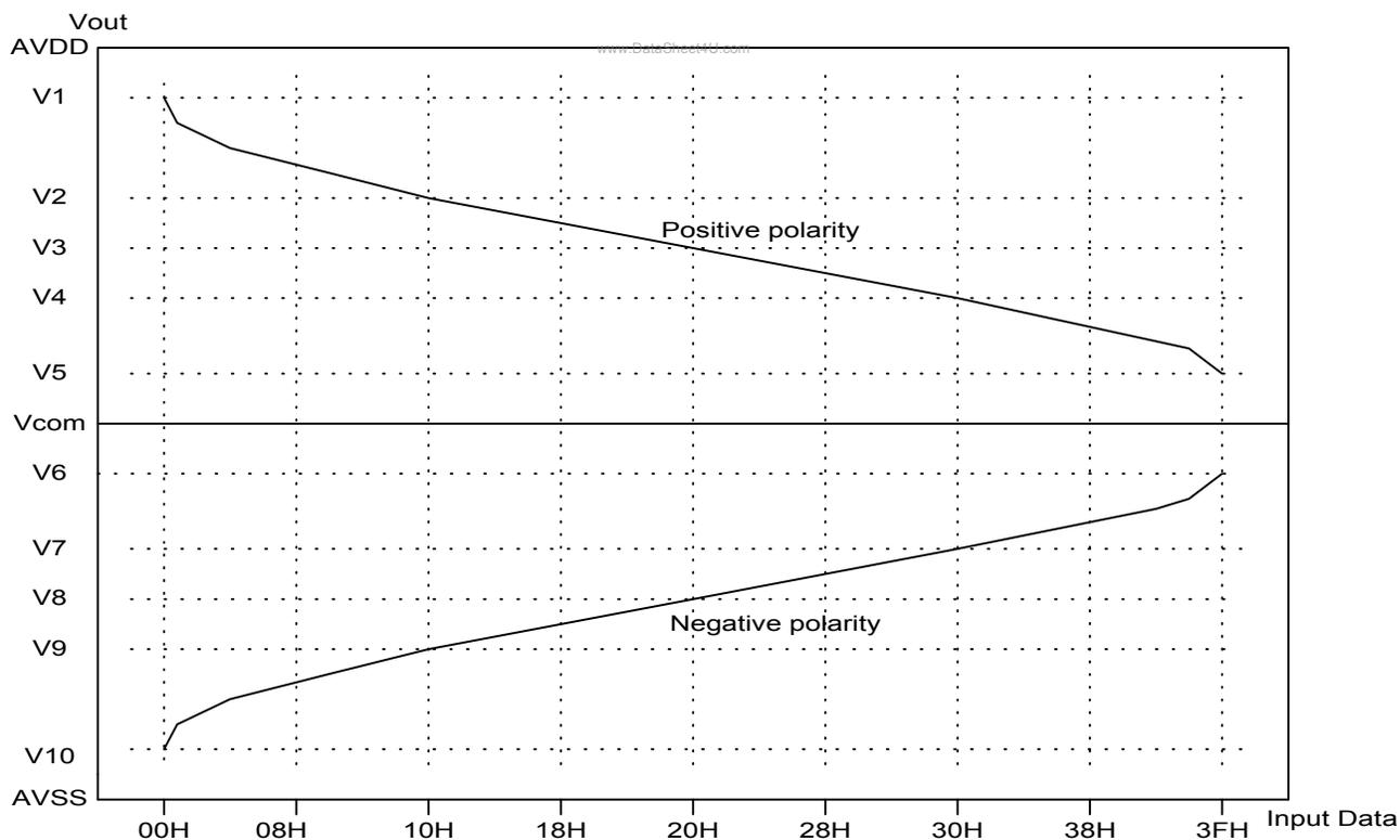
Remark :  $AVDD-0.1 \geq V1 \geq V2 \geq V3 \geq V4 \geq V5$  ;  $V6 \geq V7 \geq V8 \geq V9 \geq V10 \geq AVSS+0.1V$
