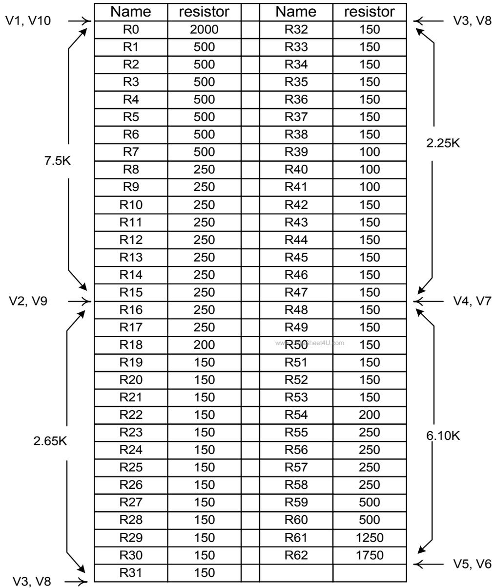
Total impedance,  $R_n=R_0 \sim R_{62}$ , equals 18.5K
