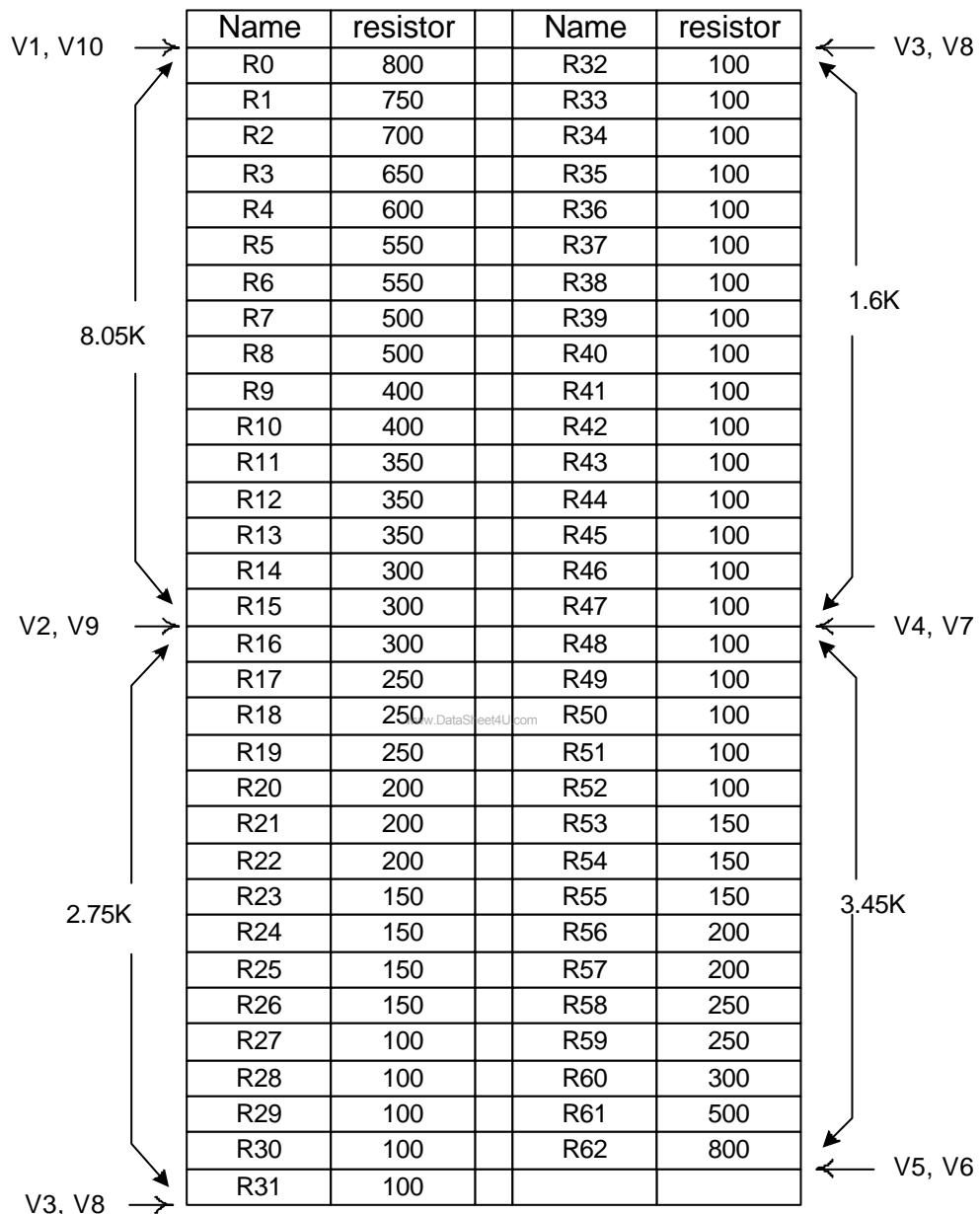
Total impedance,  $R_n = R_0 \sim R_{62}$ , equals 15.85K
