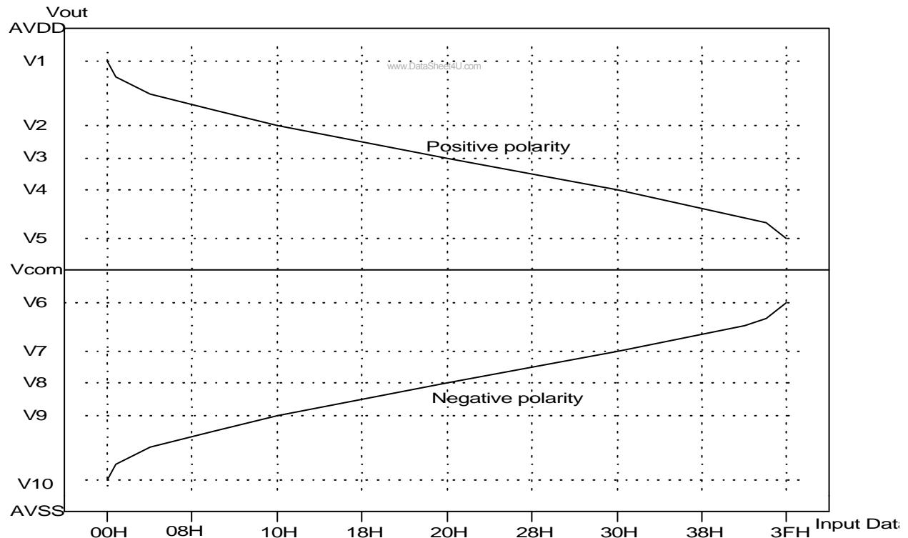
Remark: AVDD-0.1 ≥ V1 ≥ V2 ≥ V3 ≥ V4 ≥ V5; V6 ≥ V7 ≥ V8 ≥ V9 ≥ V10 ≥ AVSS+0.1V
