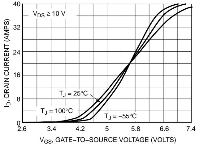
Figure 2. Transfer Characteristics
