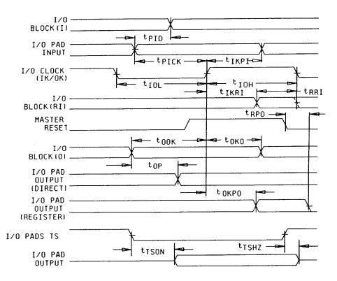
NOTE:  $t_{TSHZ}$  is determined when the output shifts 10 percent (of the output voltage swing) from  $v_{OL}$  level or  $v_{OH}$  level. See figure 5, circuit A herein for circuit used.  $t_{TSON}$  is measured at 0.5  $v_{CC}$  level with  $v_{IN} = 0.0 \text{ V}$  for three-state to active High, and  $v_{IN} = v_{CC}$  for three-state to active low. See figure 5, circuit B herein for circuit used.
