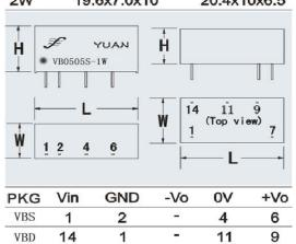
Note:PIN"7" can't connect any component.
