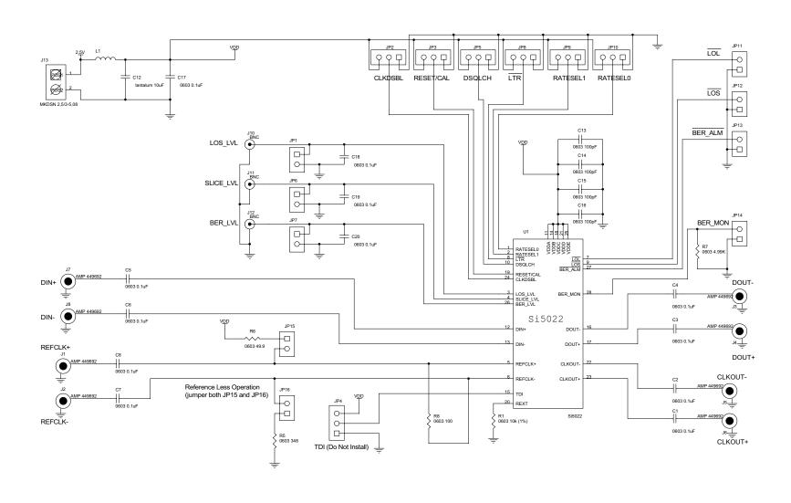
Figure 4. Si5022 Schematic
