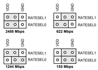
**Figure 1. RATESEL Jumper Configurations**
