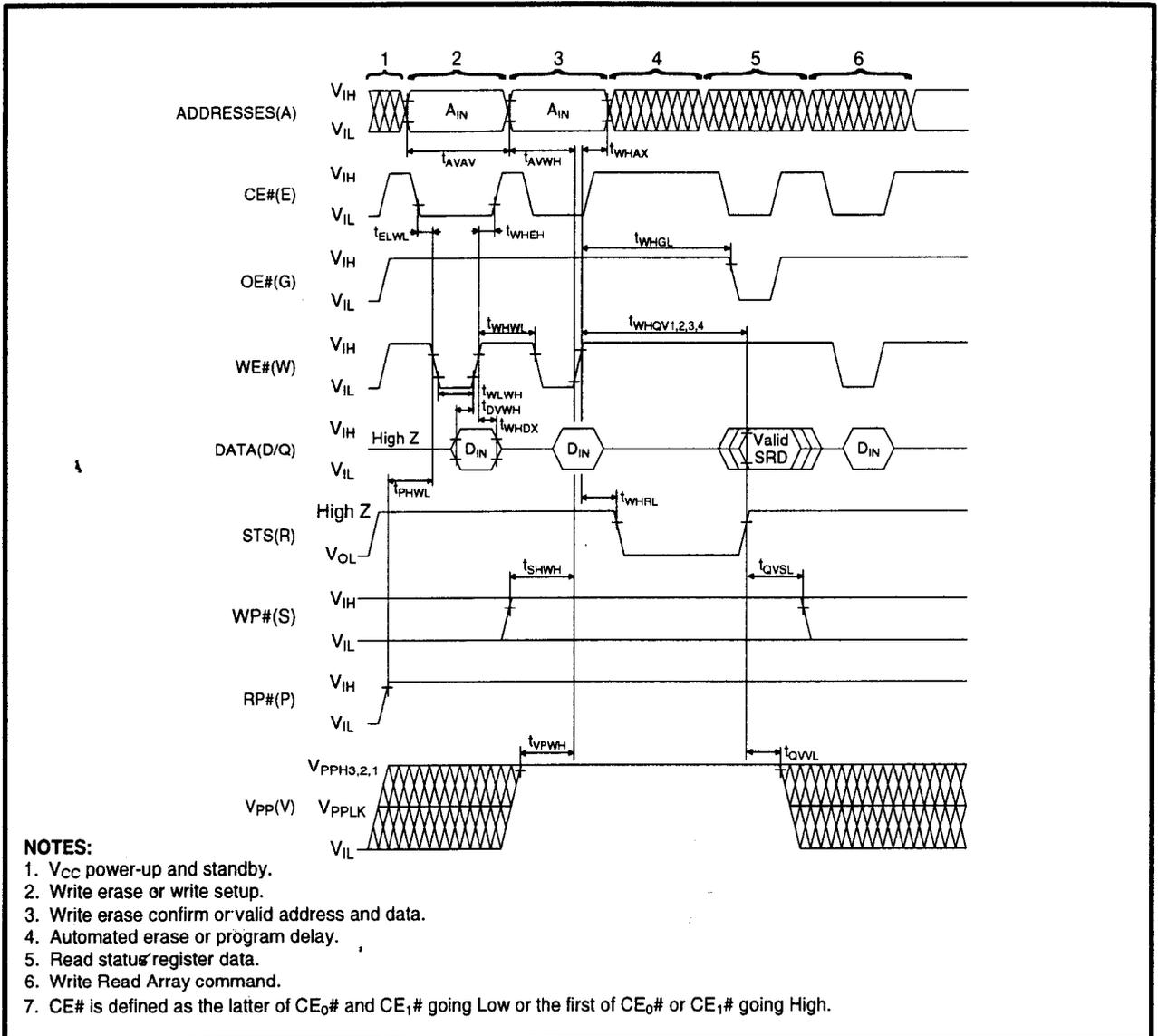
**Figure 19. AC Waveform for WE#-Controlled Write Operations**
