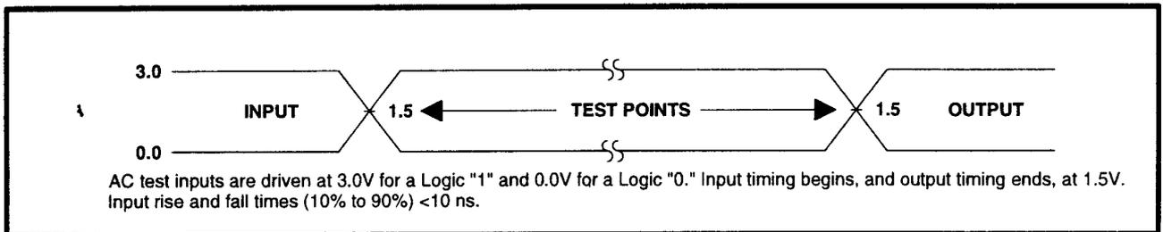
Figure 15. Transient Input/Output Reference Waveform for  $V_{CC}=3.3V\pm 0.3V$
