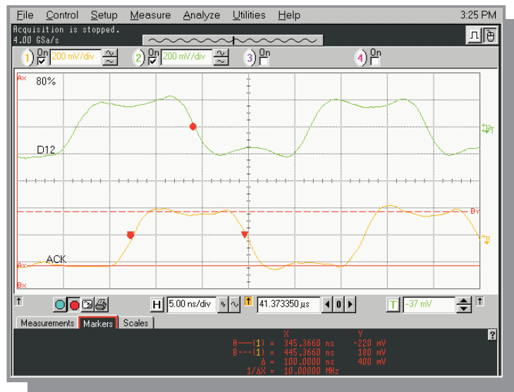
Figure C: Shows a peak-to-peak value of 400 mV for the ACK# signal with drive strength set to 80% of nominal.
