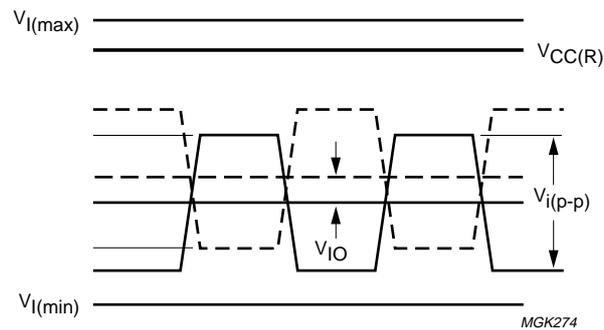
Fig.5 Logic level symbol definitions for data inputs.
