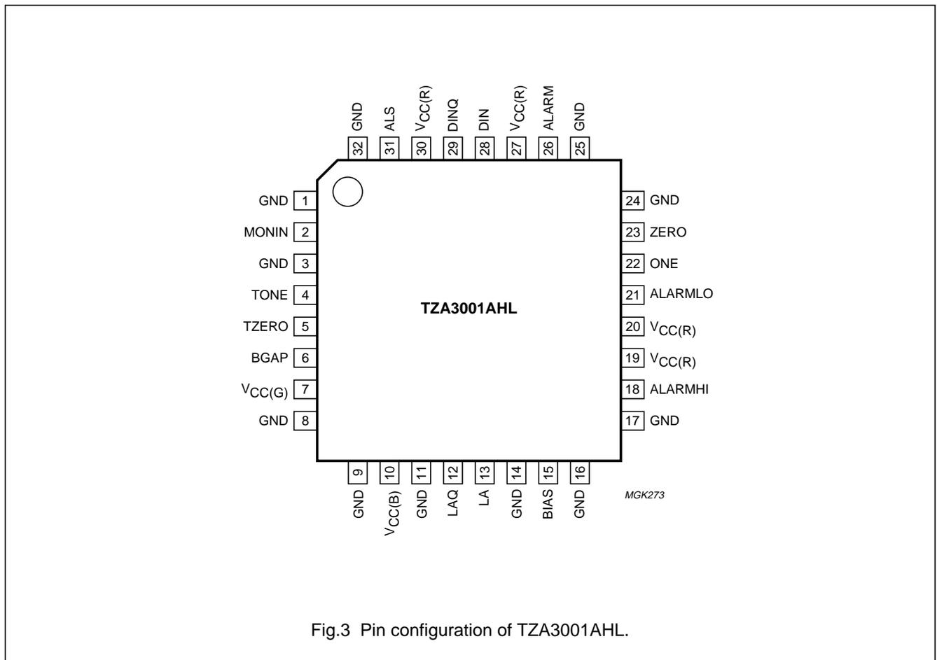
Fig.3 Pin configuration of TZA3001AHL.
