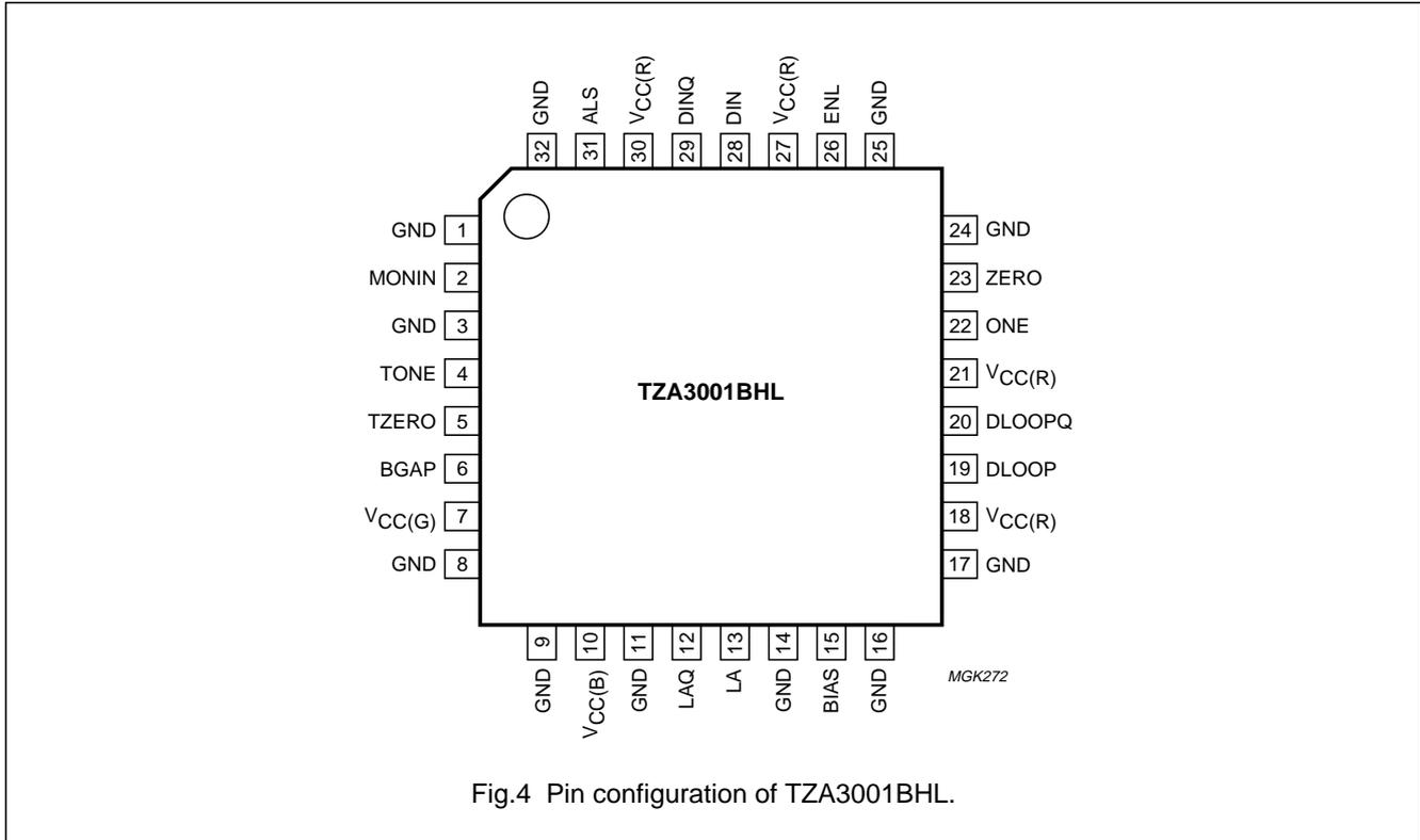
Fig.4 Pin configuration of TZA3001BHL.
