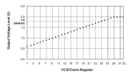
Figure 2: AAT1142 Graphical Output Voltage Programming Map.
