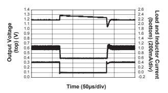
Load Transient Response (400mA to 800mA; V<sub>IN</sub> = 3.6V; V<sub>OUT</sub> = 1.0V)
