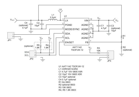
Figure 1: AAT1142 Evaluation Board Schematic.
