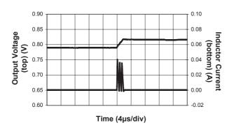
**Output Ripple** (V<sub>IN</sub> = 4.2V; V<sub>OUT</sub> = 0.8V; I<sub>OUT</sub> = 650mA)
