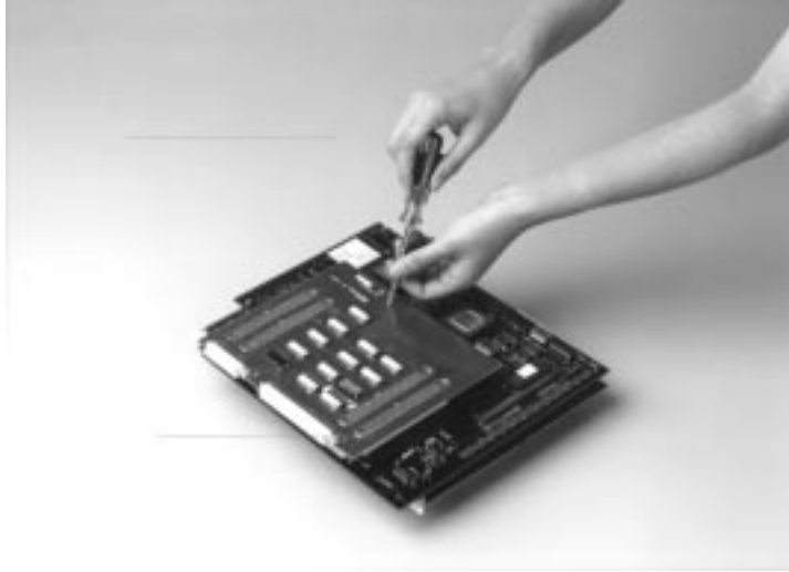
Figure 2-6. Screw Fastening of IE-75300-R-EM, IE-75000-R-BK, and Adapter Board
