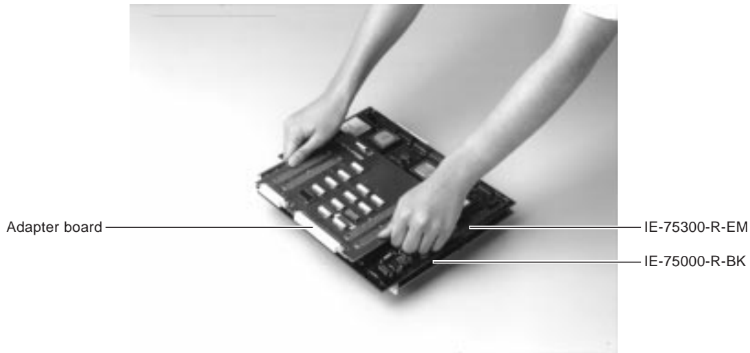
Figure 2-5. Connection of IE-75300-R-EM, IE-75000-R-BK, and Adapter Board
