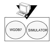
You may see that, in this case, no external hardware is required. This is the major difference between the debugging methods presently available: using a simulator or an emulator.
