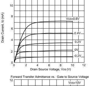
Drain Current vs. Drain Source Voltage
