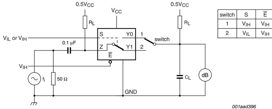
Adjust  $f_i$  voltage to obtain 0 dBm level at input.
