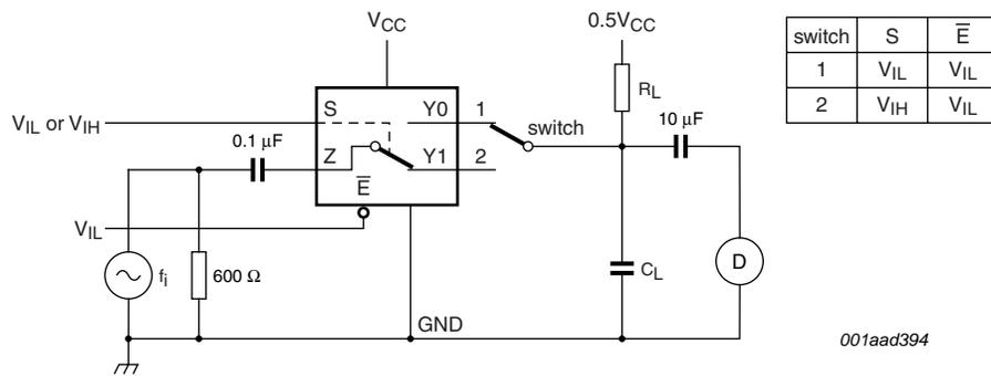
**Fig 19. Test circuit for measuring total harmonic distortion**
