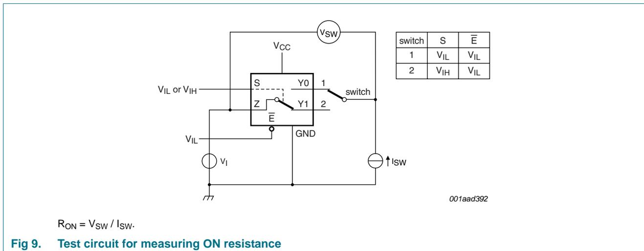
**Fig 9. Test circuit for measuring ON resistance**
