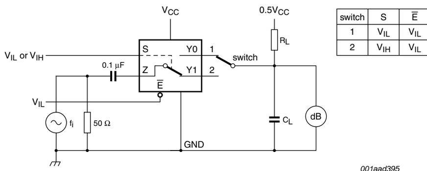
Adjust  $f_i$  voltage to obtain 0 dBm level at output. Increase  $f_i$  frequency until dB meter reads -3 dB.
