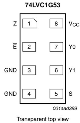
Fig 4. Pin configuration SOT833-1, SOT1089, SOT1116 and SOT1203
