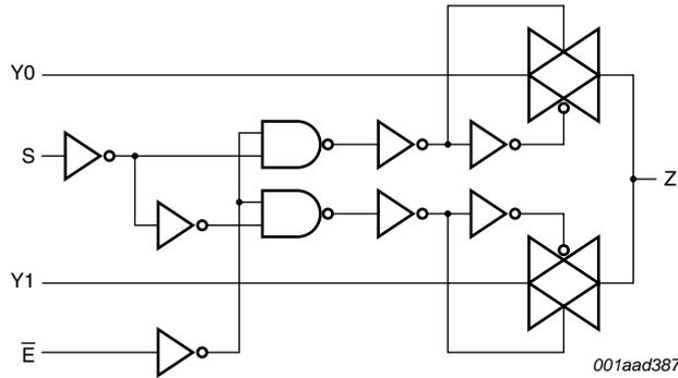
Fig 2. Logic diagram
