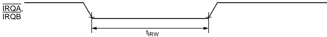
Figure 10-6 External Interrupt Timing (Negative Edge-Sensitive)
