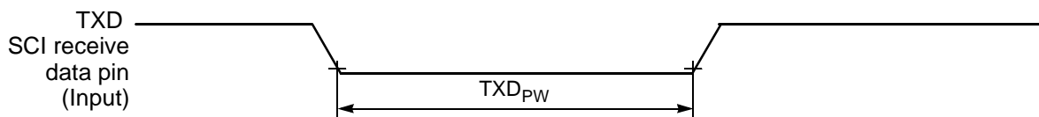
Figure 10-17 TXD Pulse Width
