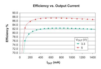
Circuit for 42 V step down to 3.3 V at 1.2 A. Efficiency data from circuit shown in left panel. Data is for reference only.
