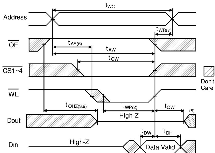
**Write Cycle No.2 Timing Waveform (1.5)**
