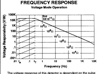
The voltage response of this detector is dependent on the pulse rate or equivalent frequency of input. The frequency response of the detector can be linearized by using a lower value resistor, but at the expense of a lower responsivity and a lower D\*. Load resistor values other than the standard 5 X 10<sup>11</sup> $\Omega$  can be specified.
