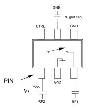
Blocking capacitors are required on all RF ports. V<sub>S</sub> can be applied at RF1 or RF2 using 10K or greater pull-up resistor.
