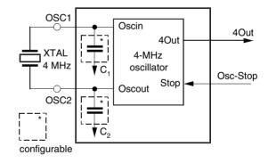
Figure 19. Ceramic Resonator
