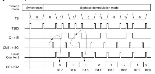
Figure 54. Bi-phase Demodulation
