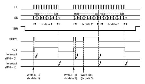
Figure 61. Example of an 8-bit Synchronous Receive Operation
