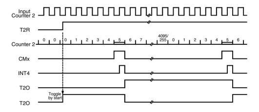
**Toggle Mode C**: A Timer 2 compare match toggles the output flip-flop (M2) →T2O
