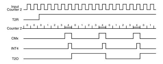
**Toggle Mode B:** A Timer 2 compare match toggles the output flip-flop (M2) →T2O
