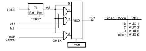
Timer 3 Demodulator for Bi-phase, Manchester and Pulse-width-modulated Signals The demodulator stage of Timer 3 can be used to decode Bi-phase, Manchester and pulse-width-coded signals
