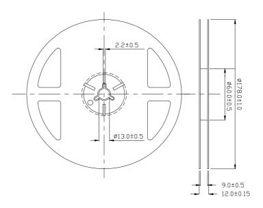
**Note:** The tolerance unless mentioned is  $\pm 0.1$ mm, unit is mm
