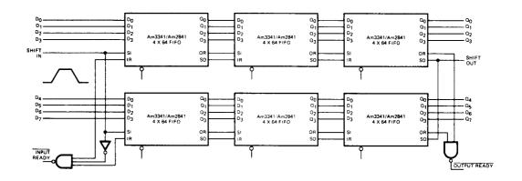
The composite input ready indicates both devices are ready to receive data. The shift in pulse must be wide enough for all devices to load data under worst case conditions.
