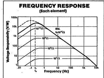
The voltage response of this detector is dependent on the pulse rate or equivalent frequency of input. The frequency response of the detector can be linearized by using a lower value resistor, but at the expense of a lower responsivity and a lower D\*. Load resistor values other than the standard  $1x10^{11}\Omega$ can be specified.
