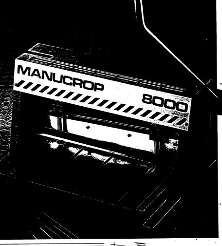
This sturdy, bench mounted, hand operated guillotine is capable of shearing 1.6mm mild steel or 3.2mm half-hard aluminium, up to a width of 508mm (20"). It can also cut sheet plastics, laminates and PCB materials. The guillotine is fully guarded, with a spring loaded work clamp holding the material in position and a built in rule to assist precision cutting. The cutting blade is reversible.
