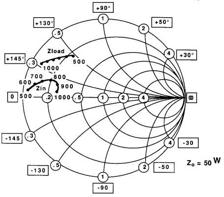
Typical series input and output impedances at rated power output conditions for single side normalized to 50 ohms.
