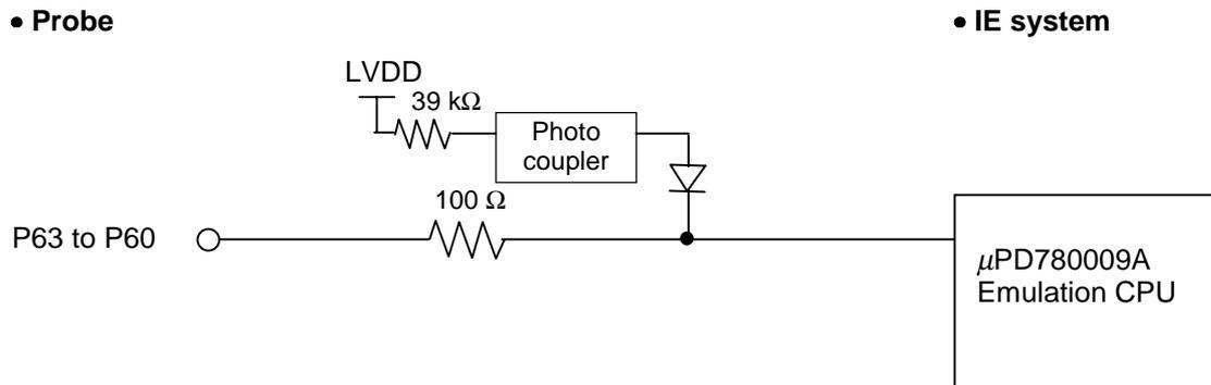
Figure 4-6. Equivalent Circuit of Emulation Circuit (c)
