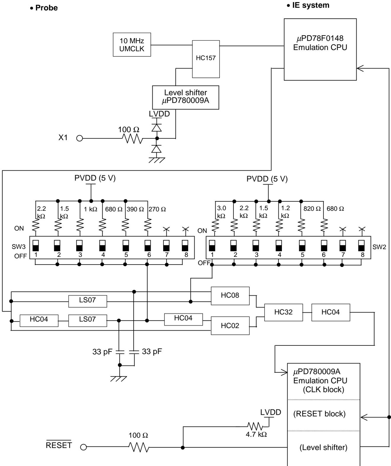
Figure 4-15. Equivalent Circuit of Emulation Circuit (c)
