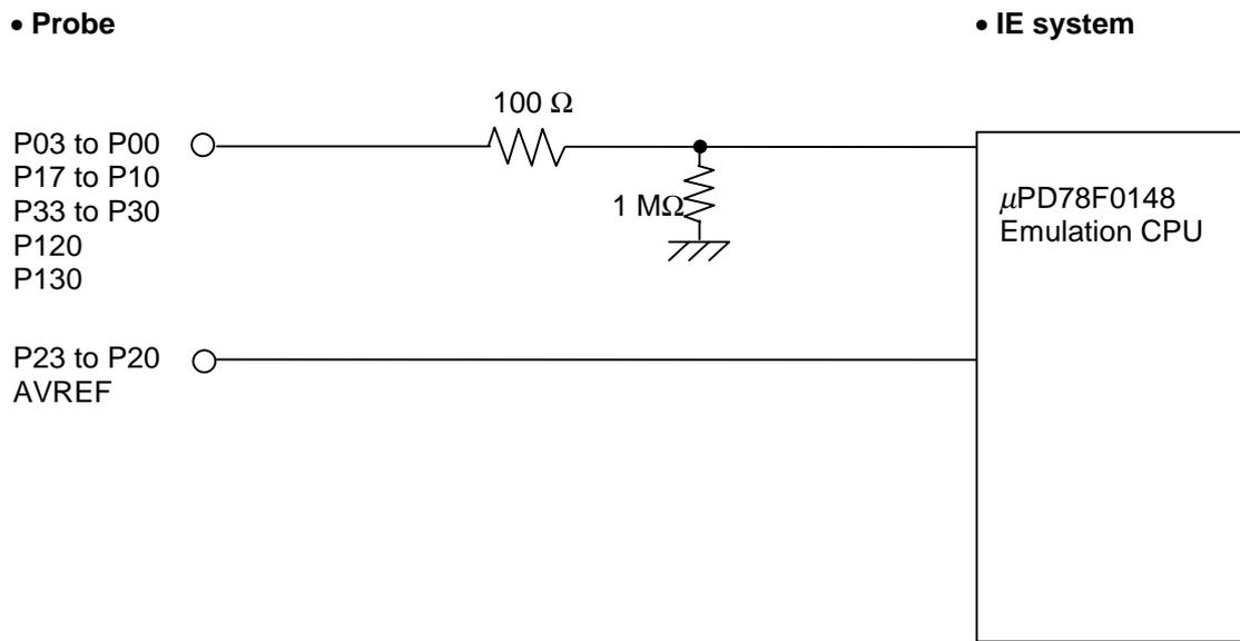
Figure 4-2. Equivalent Circuit of Emulation Circuit (c)
