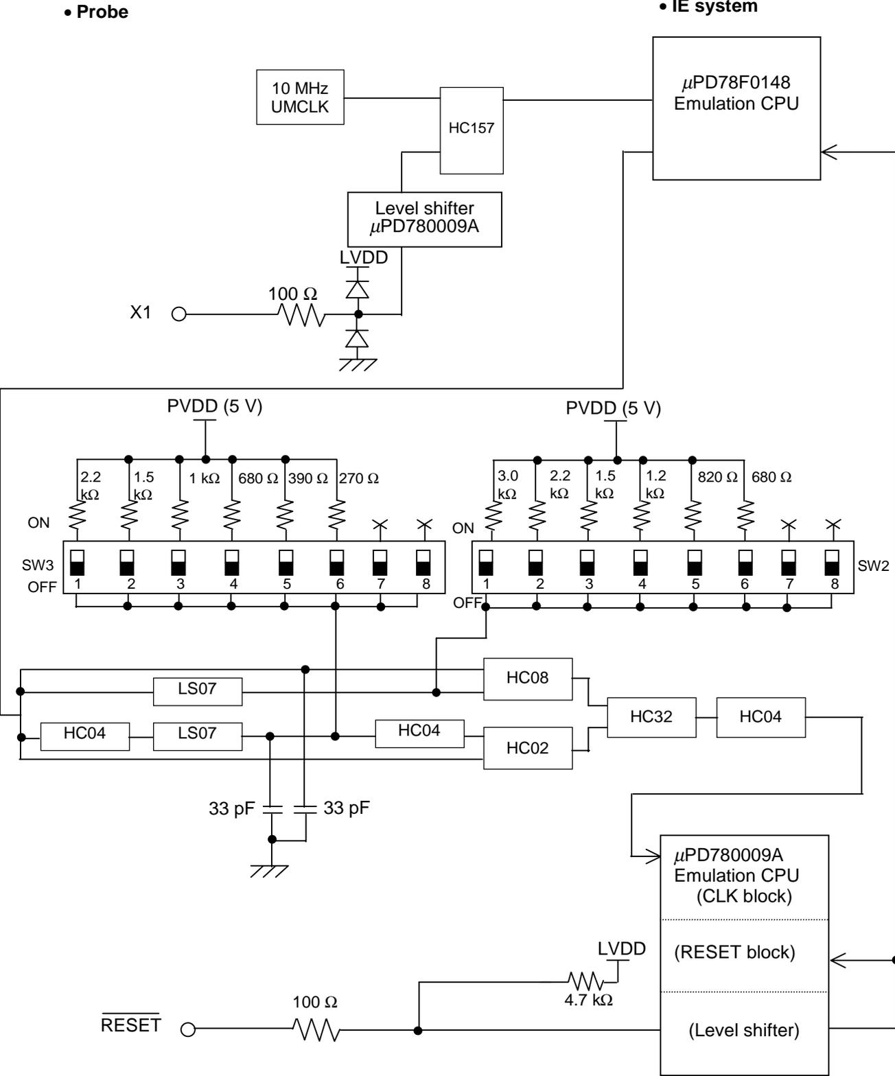
Figure 4-7. Equivalent Circuit of Emulation Circuit (c)
