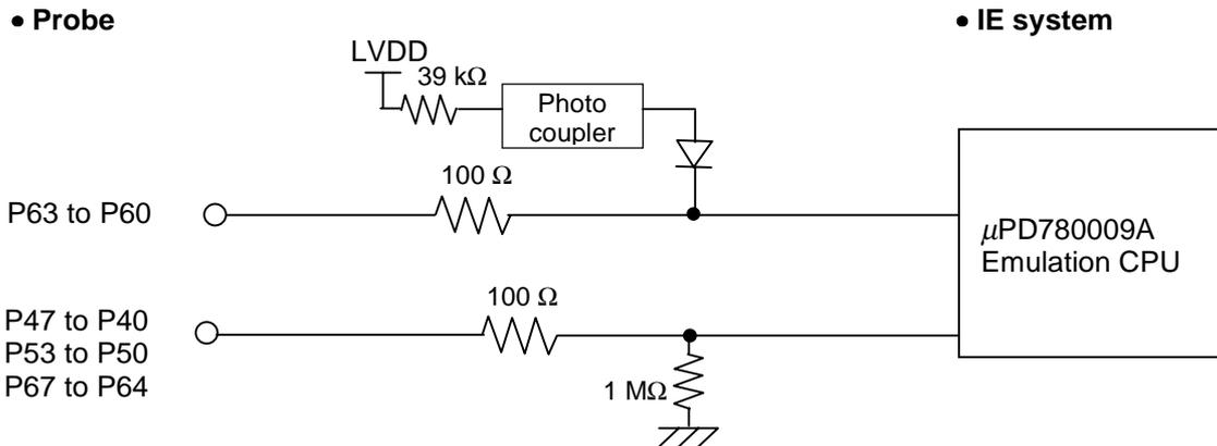
Figure 4-18. Equivalent Circuit of Emulation Circuit (c)
