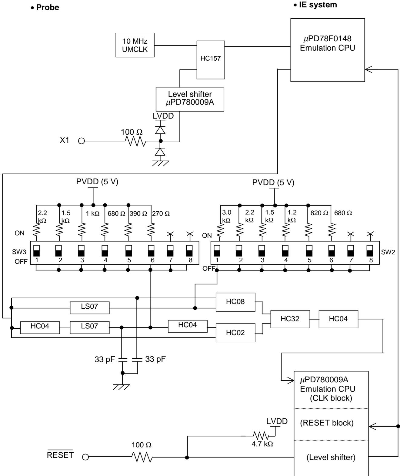
Figure 4-19. Equivalent Circuit of Emulation Circuit (c)
