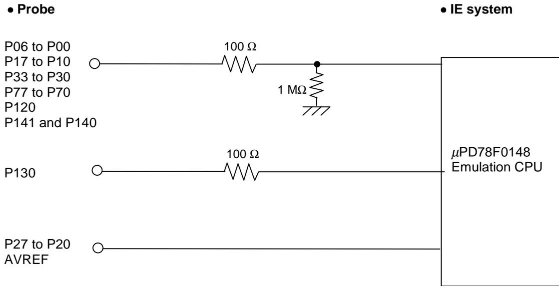
Figure 4-13. Equivalent Circuit of Emulation Circuit (b)
