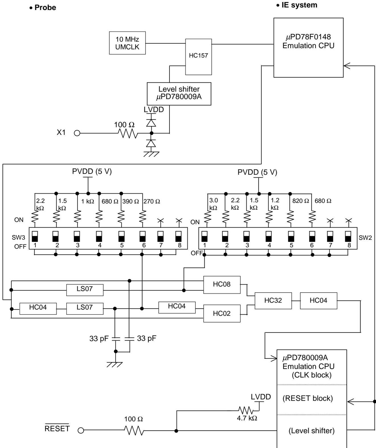
Figure 4-3. Equivalent Circuit of Emulation Circuit (c)
