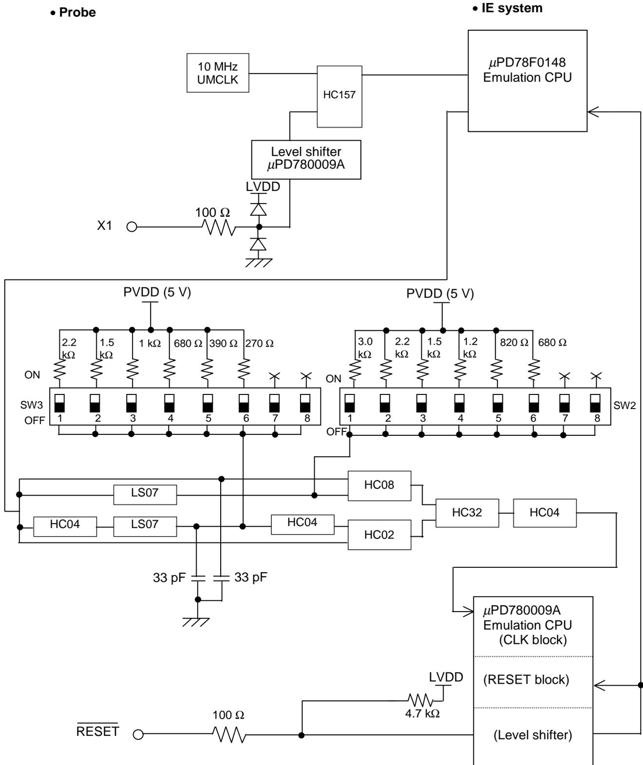
Figure 4-11. Equivalent Circuit of Emulation Circuit (c)
