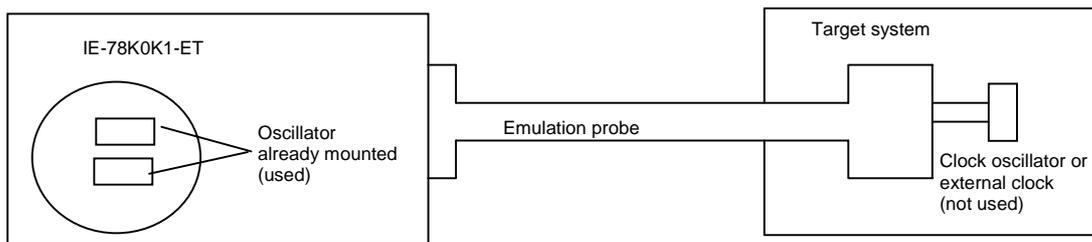
**Remark** The clock that is supplied by the IE-78K0K1-ET's oscillator (encircled in the figure) is used.
