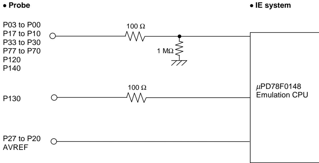
Figure 4-9. Equivalent Circuit of Emulation Circuit (b)
