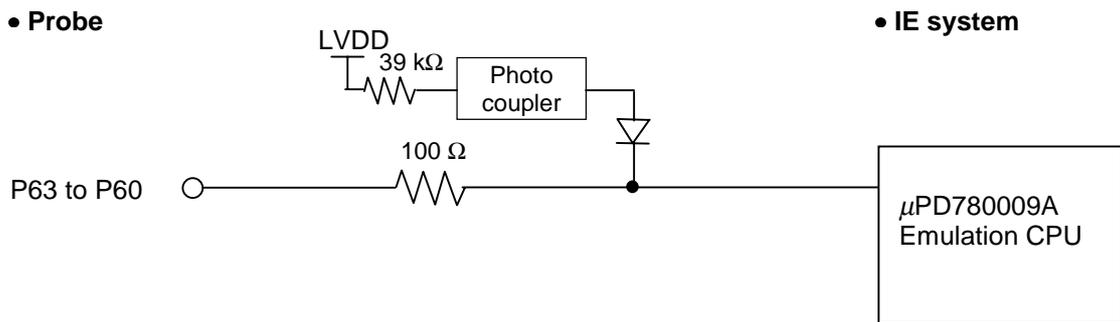
Figure 4-10. Equivalent Circuit of Emulation Circuit (c)
