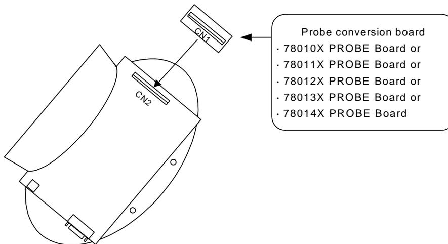
**Figure 3-2. When Not Using Probe Conversion Board**
