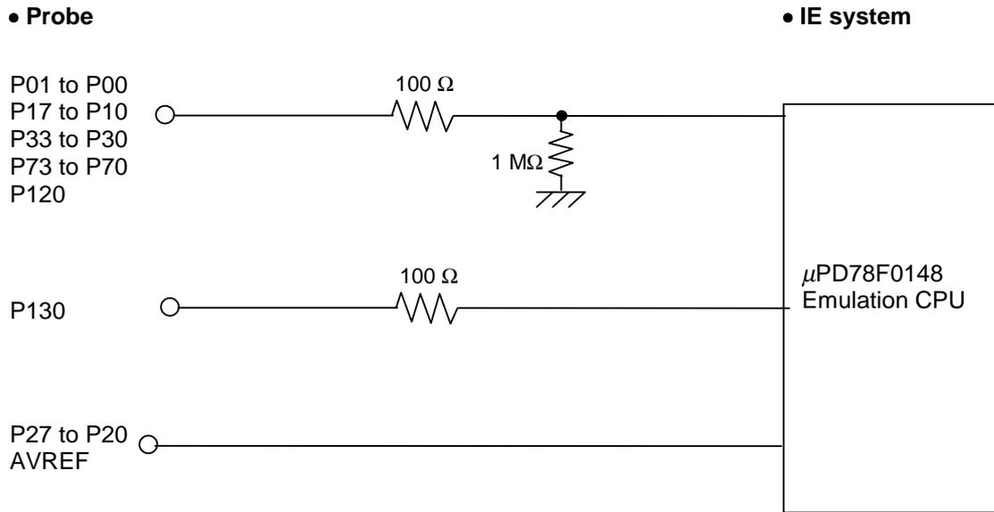
Figure 4-5. Equivalent Circuit of Emulation Circuit (b)
