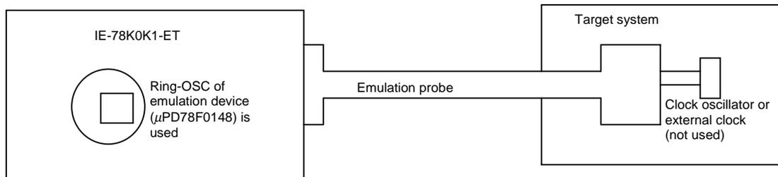
Figure 3-20. Flow of Clock (Main System Clock)
