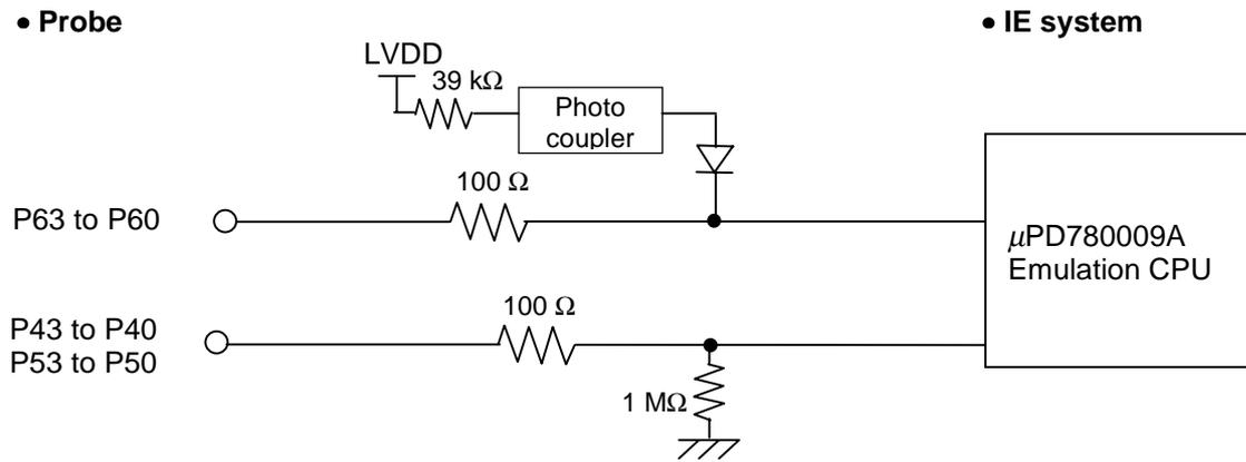
Figure 4-14. Equivalent Circuit of Emulation Circuit (c)
