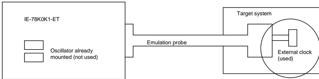
**Remark** The external clock that is supplied by the target system (encircled in the figure) is used.
