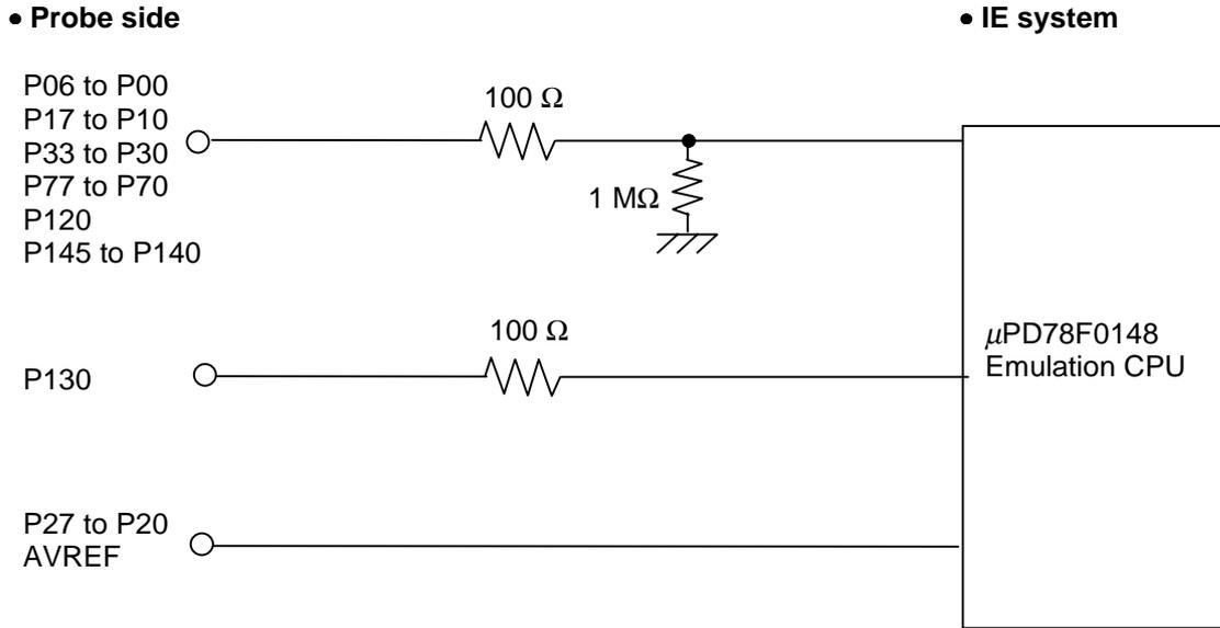
Figure 4-17. Equivalent Circuit of Emulation Circuit (b)
