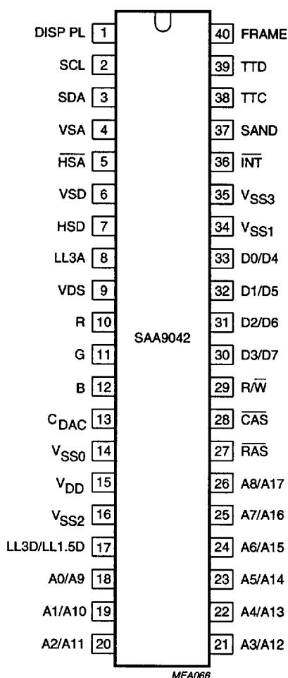
**Fig.2 Pin configuration.**
