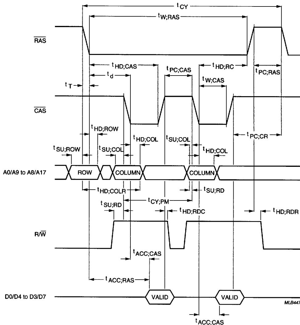
Fig.6 Memory interface timing for read cycle from external DRAM.
