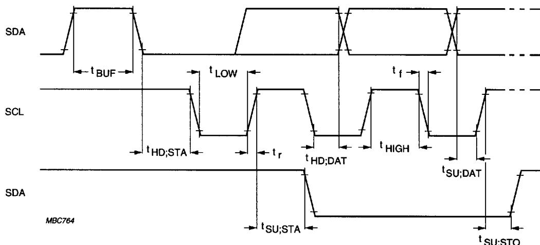
Fig.3 I<sup>2</sup>C-bus timing.
