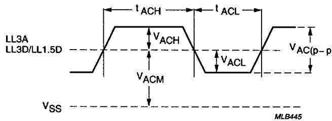
Fig.4 Line-locked system clock LL3A and LL3D/LL1.5D timing diagram.
