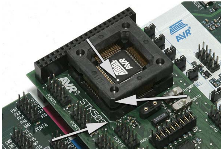
Figure 3-3: Placing the AVR in the ZIF socket.
