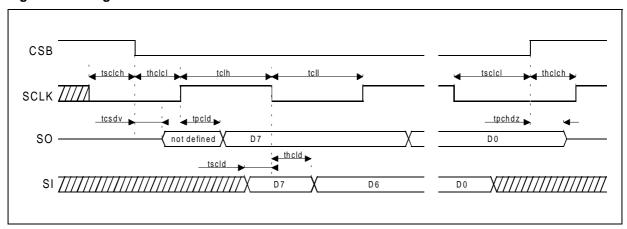
The SPI register data are transferred to the output latch at rising CSB edge. The digital filter between CSB and the output latch ensures that the data are transferred only after 8 SCLK cycles or multiple of 8 SCLK cycles since the last CSB falling edge. The CSB changes only at low SCLK.
