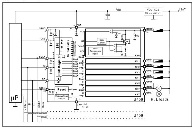
For higher current driving capability more outputs of the same kind can be paralleled. In this case the maximum flyback energy should not exceed the limit value for single output.
