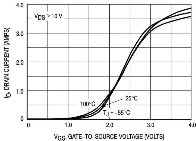
Figure 2. Transfer Characteristics
