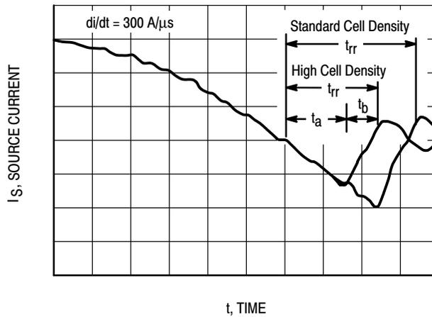
Figure 11. Reverse Recovery Time ( $t_{rr}$ )
