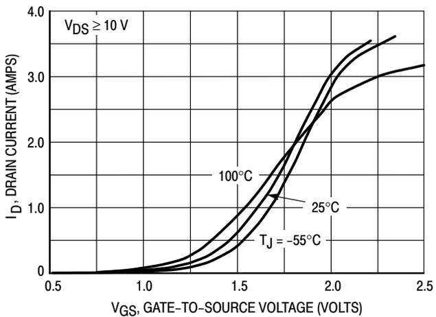
Figure 2. Transfer Characteristics
