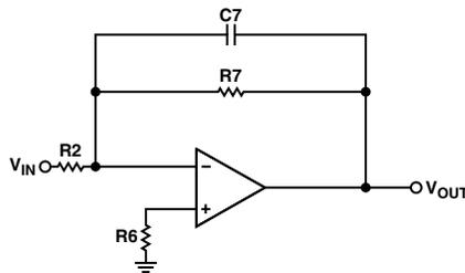
Figure 1. Simple Low-Pass Filter
