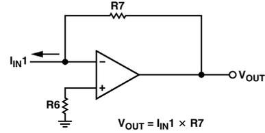
Figure 4. Current to Voltage Converter
