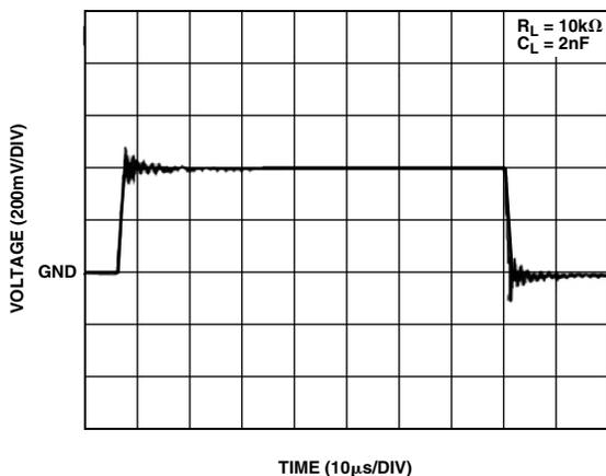
Figure 8. Capacitive Load Drive without Resistor
