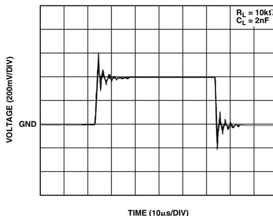
Figure 11. Capacitive Load Drive without Snubber
