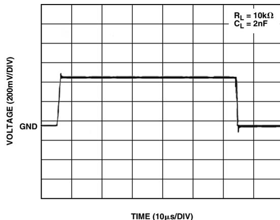
Figure 9. Capacitive Load Drive with Resistor
