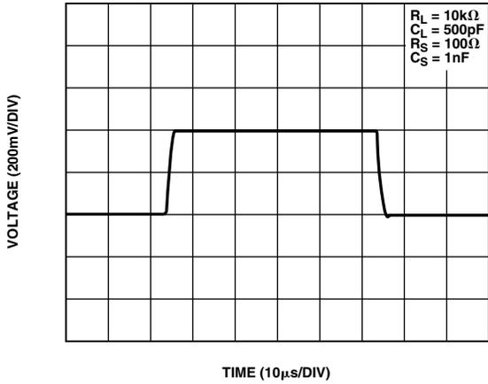
Figure 12. Capacitive Load Drive with the Snubber
