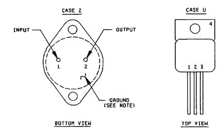
NOTE: Case is connected to ground.
