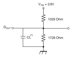
Note: Including jig and scope capacitance.
