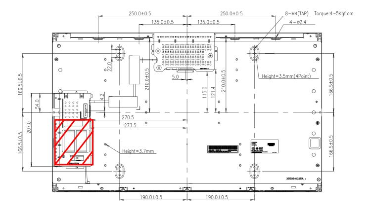
Notes : It should be recommended that any exterior materials do not go passing up the red area slanted. (For example, electrical cable, system board, etc). Otherwise, it could cause that abnormal display happens.
