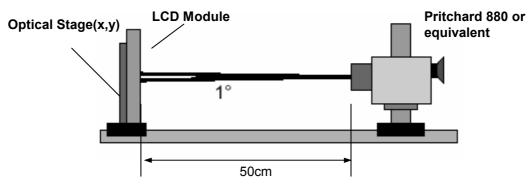
FIG. 1 Optical Characteristic Measurement Equipment and Method
