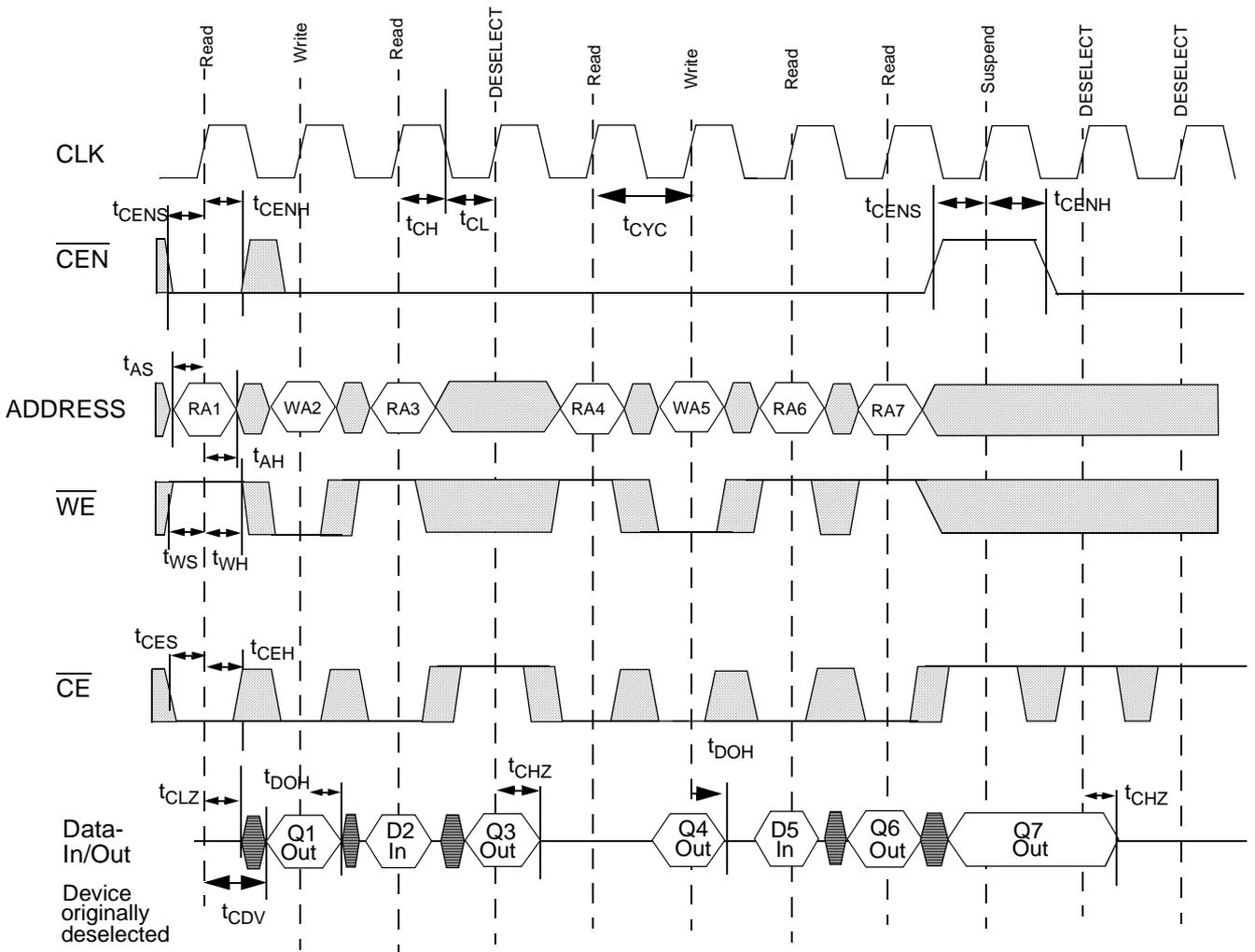
$\overline{WE}$  is the combination of  $\overline{WE}$  &  $\overline{BWS}_x$  to define a Write Cycle (see Write Cycle Description table).
