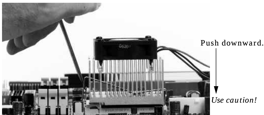
Figure 15. Pushing the Heatsink Clip Down
