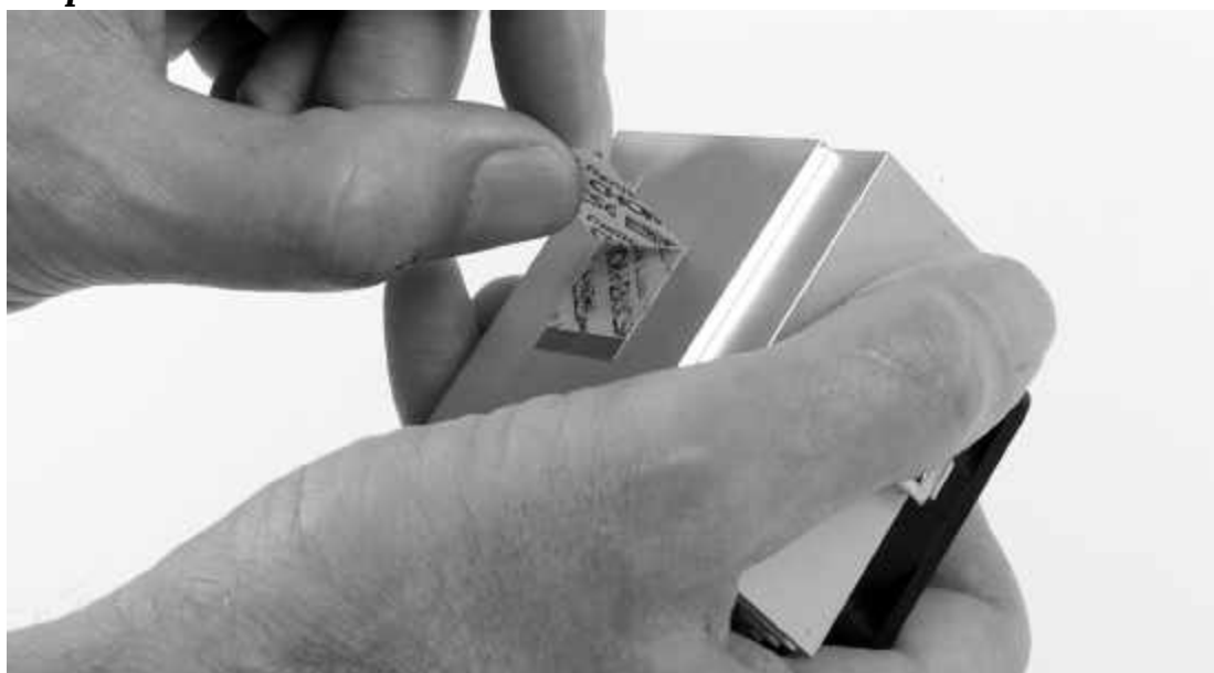
Figure 9. Pull Tape from Thermal Material with a Quick Motion
