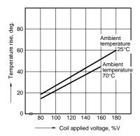
4. Ambient temperature characteristics (High capacity type)
