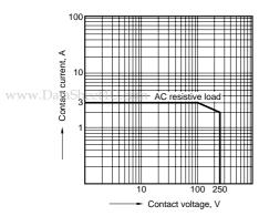
1-(2). Maximum value for switching capacity (High capacity type)
