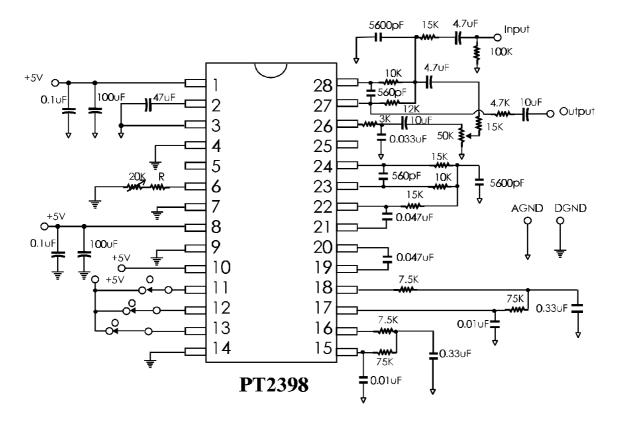
Note: External Resistor having a value of 10 K Ohms to 50 K Ohms may be used. The recommended Resistor Value (R) is 10 K Ohms. When the value of the Resistor (R) increases, the range of the Delay Time also increases.
