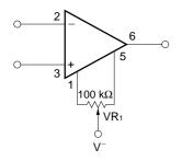
★ Remark The OFFSET NULL pins should be left open or connected to V via a resistor as shown in the left figure. Don't connect to any lines other than V, otherwise mulfunction, degradation, or failure may occur.
